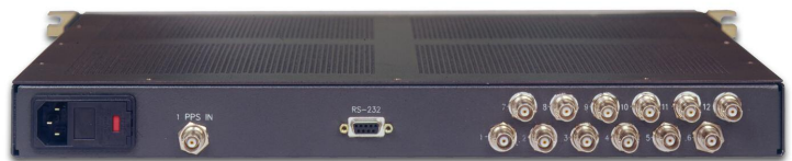
8040C connections (shown with 12 output option)
